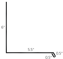
Side Wall Flashing with Hem (SWFH)
